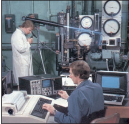
High-intensity illumination and fiber optic boroscope enables research scientists to view valve action in compressor while it is running.
