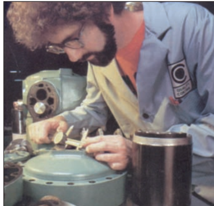
Randomly selected units are taken from the production run and totally disassembled for a thorough on-going quality evaluation.
